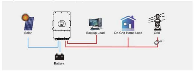
Hybrid inverter will not only provide power to the backup load connected but also give power to the home load connected. If PV power and battery power is insufficient, it will take grid energy as supplement. The hybrid inverter will not sell power to grid. The external CT(&Meter) will detect power flowing back to the grid and will reduce the power of the inverter only to supply the local load, charge battery and home load. This control is achieved by:
