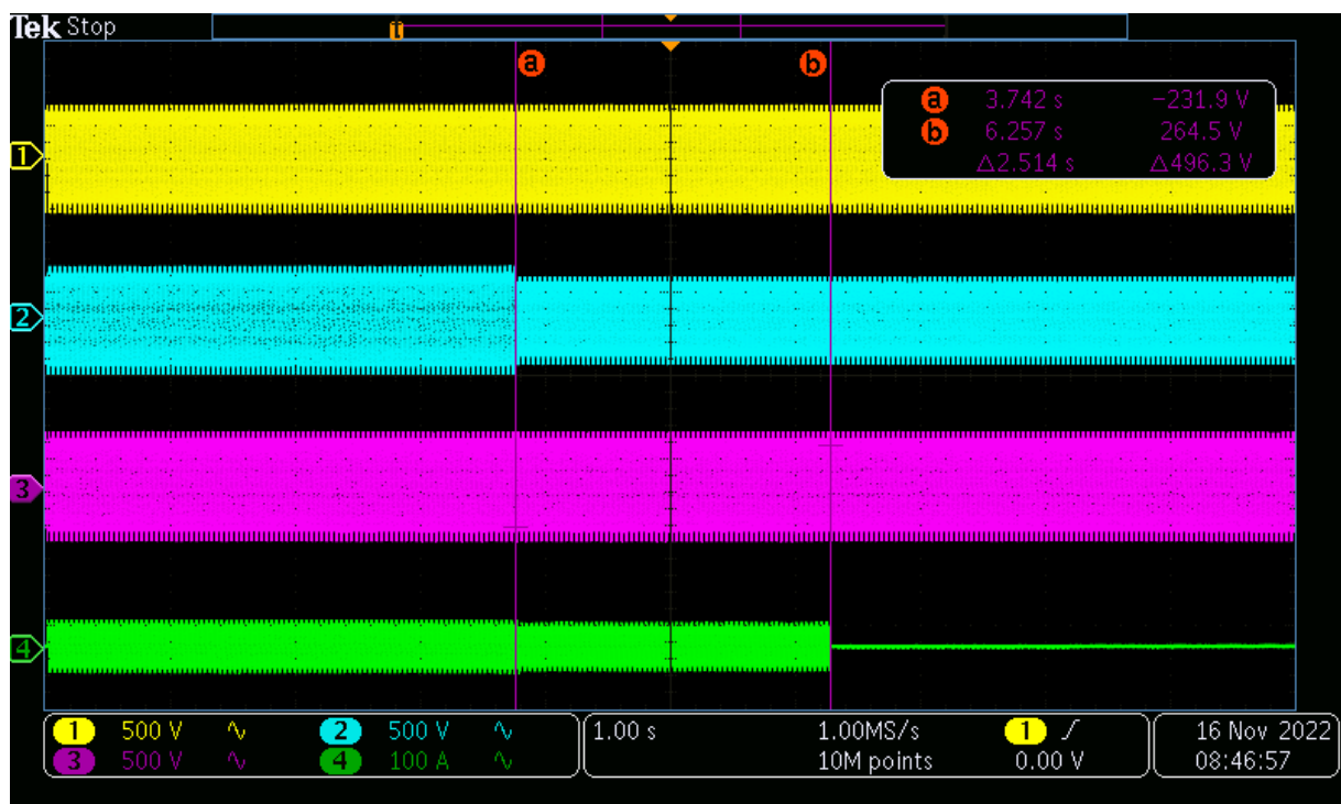
Figure 10 – Test U/V (Trip test, L2-N)
