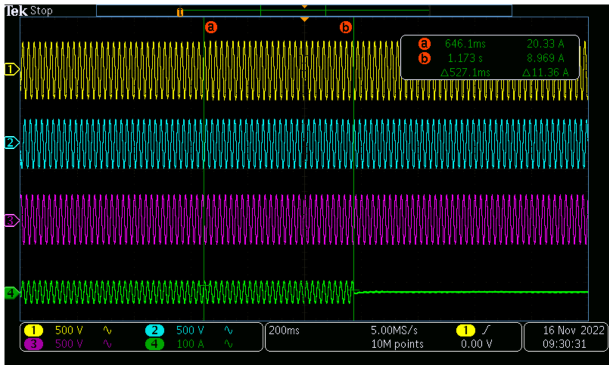
Figure 15 – Test O/V stage 2 (Trip test, L1-N)
