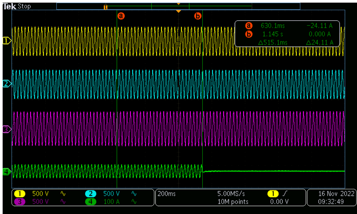
Figure 17 – Test O/V stage 2 (Trip test, L3-N)
